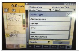
**Press** on **DGPS Type** and Select the Type of Correction – 'RTK'
